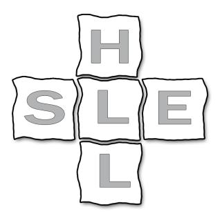
In this model the match or mismatch of the blocks (interface) is just as important as the characteristics of the blocks themselves. A mismatch can be a source of human error. It should be mentioned that this building block diagram is only intended as a basic aid to understanding Human Factors.
